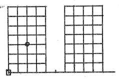
When  $i\ge 0$ , the point X,Y represents the lower, left hand corner of the box (squared in the diagram) of the first character. When i<0, the point X,Y represents the point circled in the diagram. The latter point is the "center" of the box (for i<0); furthermore, the drawing of these characters begins and ends at that point for  $-10\le i\le -2$ . Thus, the characters produced for  $-10\le i\le -2$  are well suited to mark specific points of lines or curves.
